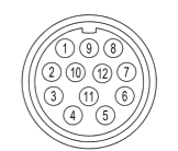
H connector (12 pin) - M23 CCW Hummel 7.410.000000 - 7.002.912.603 solder side view FV
